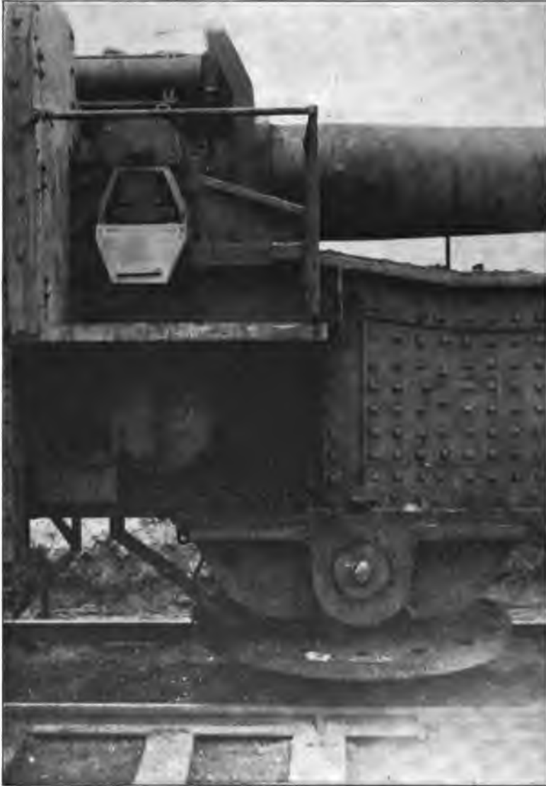
CENTER PIVOT, ELEVATING WORM, AND ANTI-FRICTION BEARING OF THE 210-MM. GERMAN GUN MOUNT.
